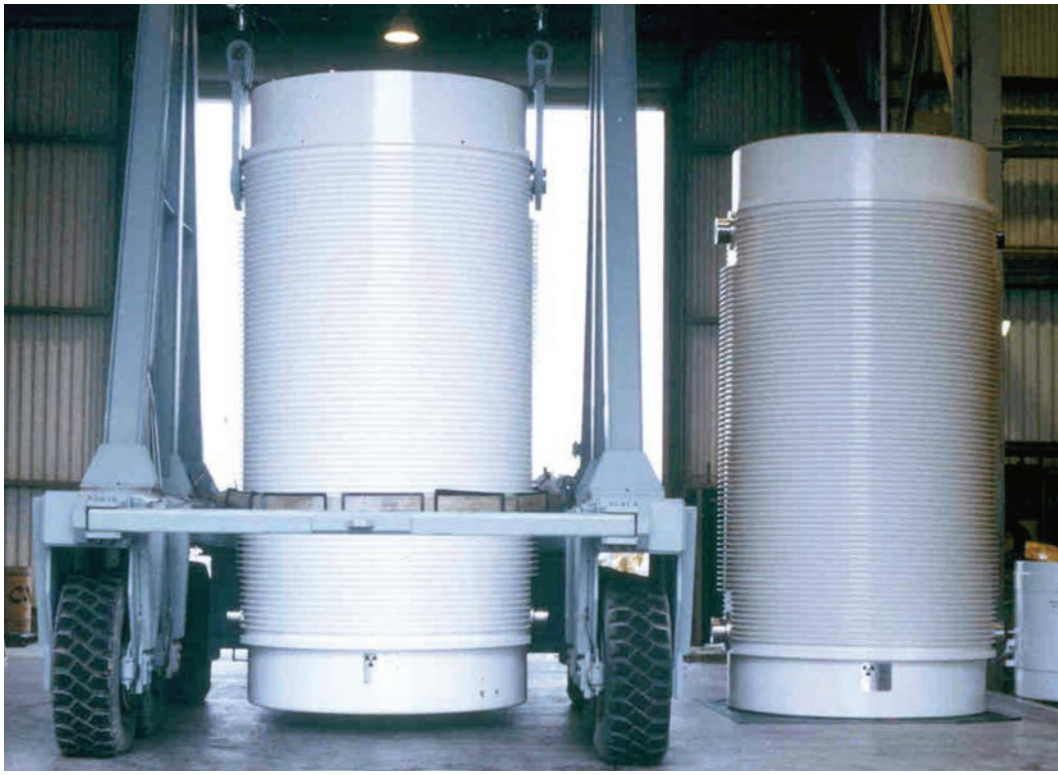
FIGURE 3.3. A spent fuel cask being transported at the Surry nuclear plant in Virginia. A typical dry storage cask is approximately 18 feet tall and can weigh up to 350,000 pounds when fully loaded.
